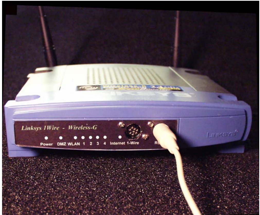
Figure 2 – Finished LINKSYS WRT54GS with LP-LINKSYS-1W adapter installed inside a modified case (for the 2 new connectors) and a new label installed.
