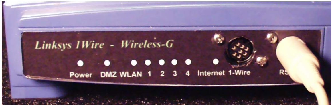
Figure 8 – note the location of the mini-din screws
